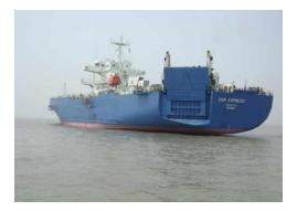
Type of Vessel:RoRo-PCC (Pure Car Carrier)Completely Reconstructed to PCC:January 2009Built:1991Speed:abt. 20 Kn.Loading Capacity:abt. 650 Private CarsThe vessel is in excellent condition; Practically a New Building
